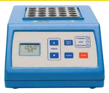
The Analytical 3980 COD reactor is an easy to use test tube heater. Its well-marked user interface provides intultive operation. the reactor is equipped with tow predefined temperature settings: 150° and 105°C. COD and total phosphorus digestions are conducted at 150°C, and total nitrogen digestions are at the 105°C.
